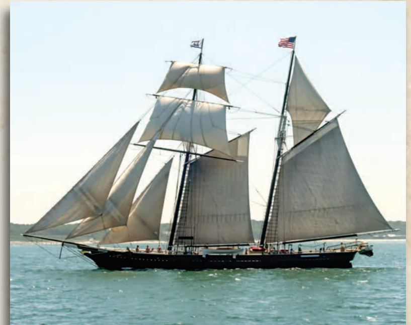
Typical Schooner, a ship with at least two masts, with the foremast smaller than the mainmast.
